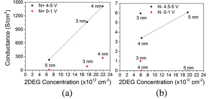
Figure 5: Linear fit of conductance plotted against 2DEG concentration for (a) N+ and (b) N- GaN.
