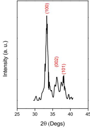
Figure 4: XRD plot of AlN on Si(100). Polarization strain is indicated by the 002 orientation.
