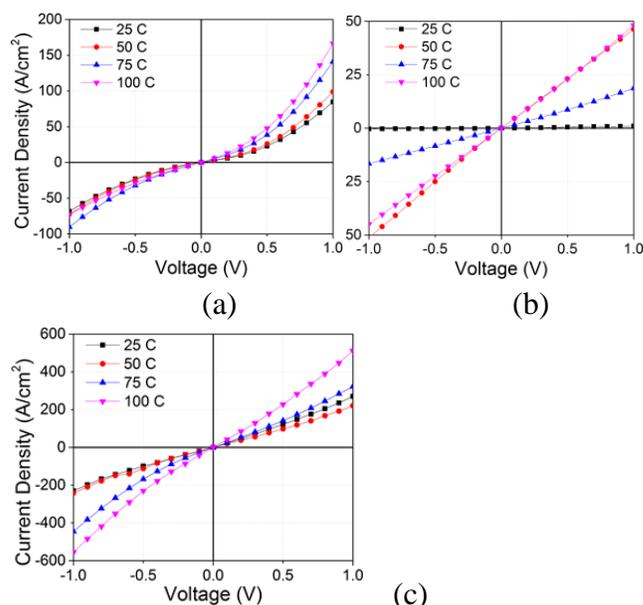
Figure 3: Temperature-dependent JV plots of (a) 3 nm AlN on N+ GaN, (b) 3 nm AlN on N- GaN, and (c) 4 nm AlN on N+ GaN
