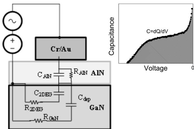
Figure 1: Schematic of the AlN/GaN MOSCAP along with plot of reverse bias integration method to determine 2DEG.
