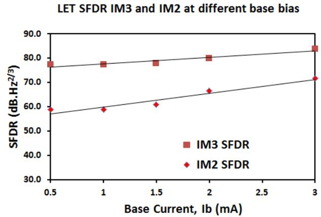
Figure 3: SFDR for IM3 and IM2 of LET at different base current bias ( $I_B$ ).
