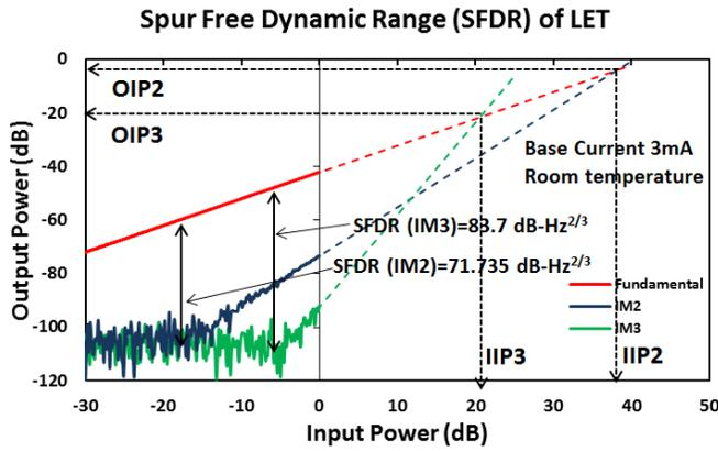
Figure 2: (a) Two tone 0.995 and 1.005GHz spur free dynamic (SFDR) measurement of LET at base current bias ( $I_B$ ) 3mA.
