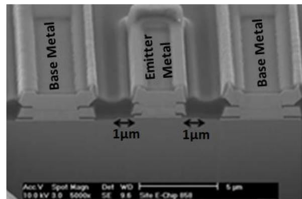
Figure 1: Scanning electron microscope photomicrograph showing the cross section of the LET.
