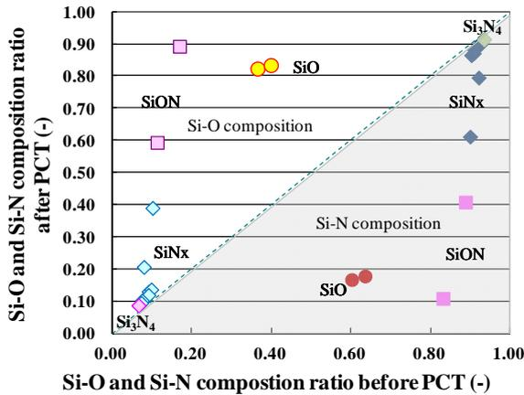
Fig. 2 The Si-O and Si-N composition ratio before/after PCT
