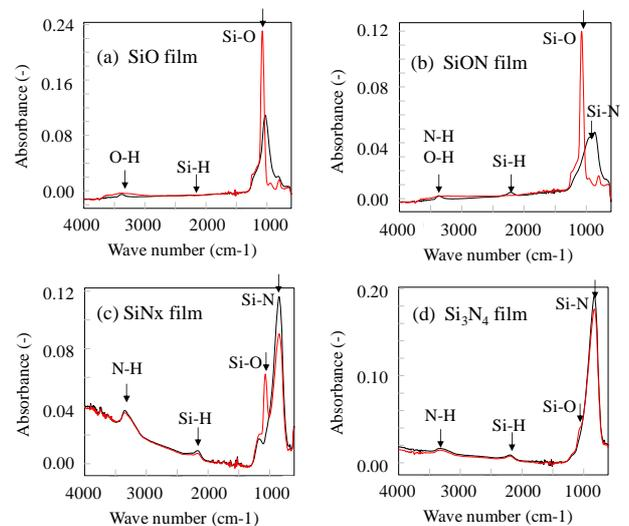
Fig. 1 FTIR absorption spectra for (a) SiO films, (b) SiON films, (c) SiN<sub>x</sub> films prepared by PECVD and (d) Si<sub>3</sub>N<sub>4</sub> films deposited by Cat-CVD before (black spectra) and after PCT (red spectra)
