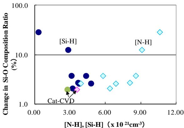
Fig. 3 The oxidation of the silicon nitride films by PCT
