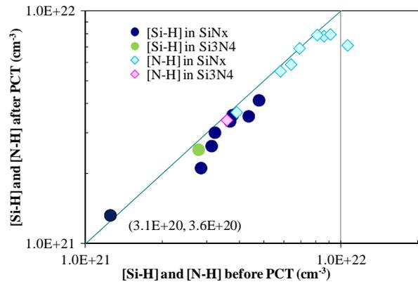
Fig. 4 The densities of Si-H and N-H bonds in the silicon nitride films before and after PCT
