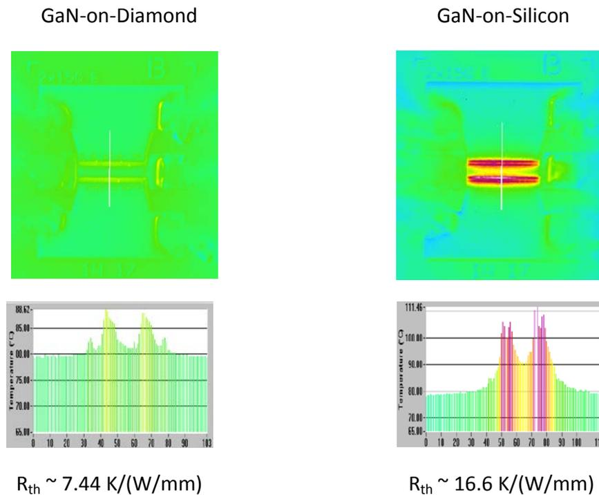
Figure 1. IR images of GaN/Diamond and GaN/Si devices.  $R_{th} \sim (T_{peak} - T_{base}) / (V_d * I_d)$ . Representative  $R_{th}$  for GaN/SiC is 11.5 K/(W/mm).
