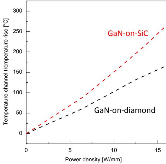
Figure 1: Peak channel temperatures obtained for  $2 \times 100 \mu\text{m}$ ,  $35 \mu\text{m}$  gate pitch AlGaIn/GaN HEMTs, comparing GaN-on-diamond versus GaN-on-SiC. The GaN-on-diamond transistor exhibits a 40% lower thermal resistance for the measured device geometry. Peak channel temperature was determined from Raman thermography measurements with the aid of thermal modeling.
