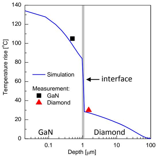
Figure 3: Measured GaN and diamond temperatures for a  $4 \times 100 \mu\text{m}$ ,  $35 \mu\text{m}$  gate pitch GaN-on-diamond transistor operated at a 17.5 V source drain bias and 11.4 W/mm power dissipation. The vertical temperature profile overlaid is generated from a 3-D finite element model, using thermal material parameters determined experimentally.
