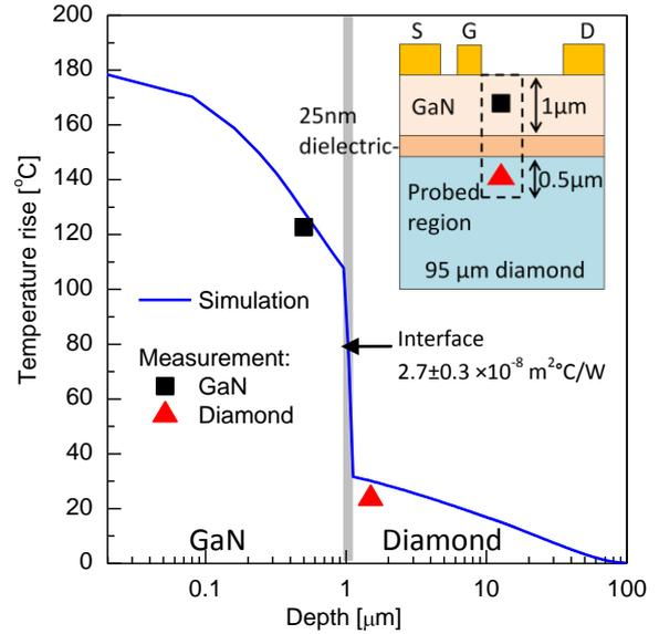
Figure 2: Measured GaN and diamond temperatures for a  $2 \times 100 \mu\text{m}$ ,  $35 \mu\text{m}$  gate pitch GaN-on-diamond transistor operated at a 20 V source drain bias and 15.7 W/mm power dissipation. A schematic cross section of area probed in the Raman measurement is shown as an inset. The vertical temperature profile overlaid is generated from a 3-D finite element modeling, using thermal material parameters determined experimentally.
