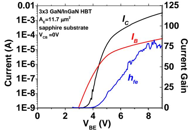
Figure 2. The Gummel plot of a GaN/InGaN HBT using the Pd-based contact scheme.
