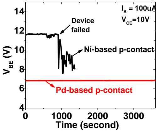
Figure 1. A chart showing the evolution of  $V_{BE}$  under a constant  $I_B$  stressing condition in the forward active mode. The devices under test have  $A_E = 20 \times 20 \mu\text{m}^2$  and  $I_B = 100 \mu\text{A}$  at  $V_{CE} = 10 \text{ V}$ .
