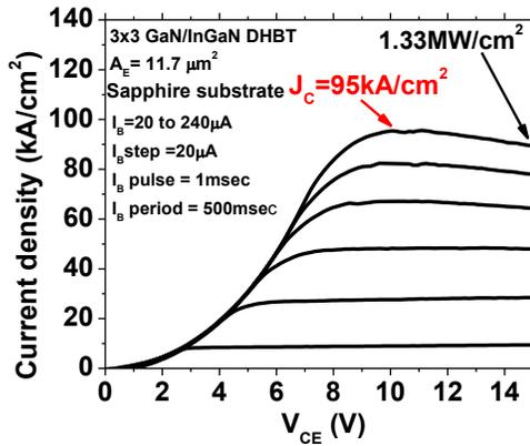
Figure 3 The quasi-static common-emitter family curves of a GaN/InGaN HBT using a Pd-based p-type base contact scheme.
