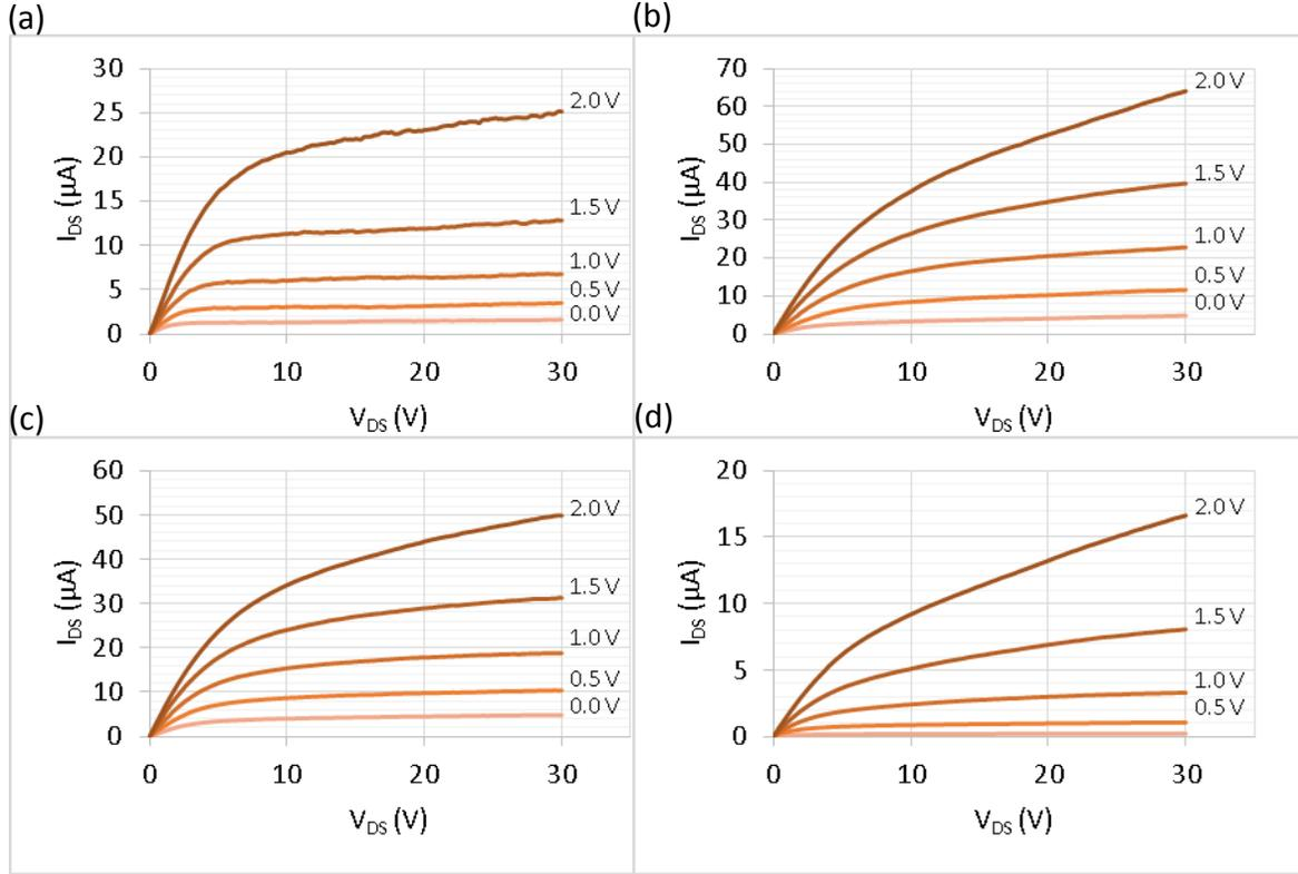
Fig. 2. Output characteristics of the ZnO SGTFTs for a gate-to-drain spacing of (a) 9  $\mu\text{m}$ , (b) 16  $\mu\text{m}$ , (c) 23  $\mu\text{m}$ , and (d) 30  $\mu\text{m}$ .
