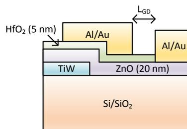
**Fig. 1.** Cross-section schematic image of the ZnO SGTFT.
