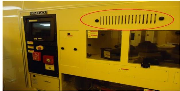
Figure 9. Plating cabinet and louvers to block air flow (circled).
