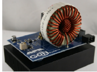
Figure 1: A 5KW boost converter based on GaN HEMTs. At 1MHz, nearly 97% efficiency can be achieved at 2.3KW. Courtesy APEI Inc.
