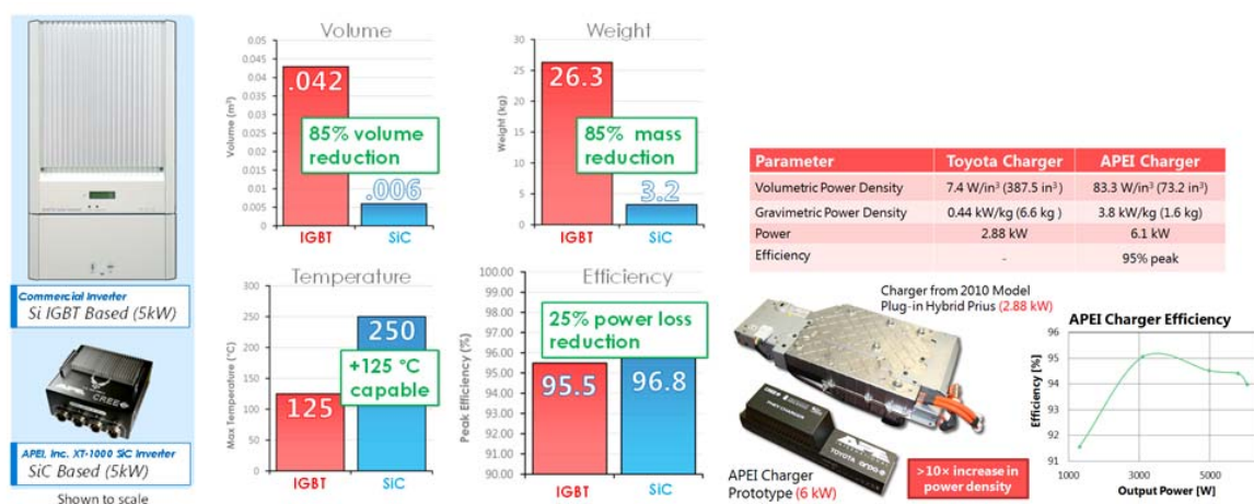
Figure 2: A compact 5KW inverter based on SiC MOSFETs, offering compelling improvements, valuable for applications such as avionics. The higher semiconductor cost is also offset by the BOM cost and operating cost reductions. A 6KW battery charger using SiC, with much improved power density. Courtesy APEI & Cree Inc.
