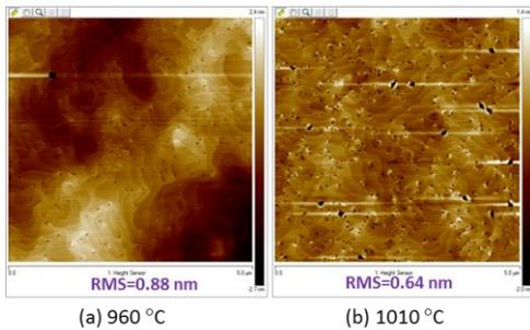
Fig. 2 5 μm x 5 μm AFM images of AlGa<sub>N</sub>/GaN heterostructures in H<sub>2</sub> ambient, (a) 960 °C, (b) 1010 °C.
