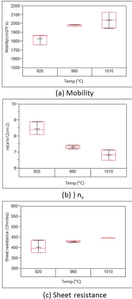
Fig. 5 Electrical properties of the AlGaIn/GaN heterostructures in  $N_2$  ambient at 920 °C, 960 °C and 1010 °C. (a) Mobility, (b) Sheet carrier concentration  $n_s$ , (c) Sheet resistance.
