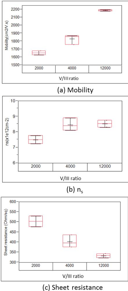
Fig. 7 Electrical properties of the AlGaIn/GaN heterostructures grown at 920 °C with different V/III ratios (2,000, 4,000, and 12,000), (a) Mobility, (b) Sheet carrier concentration n<sub>s</sub>, (c) Sheet resistance.
