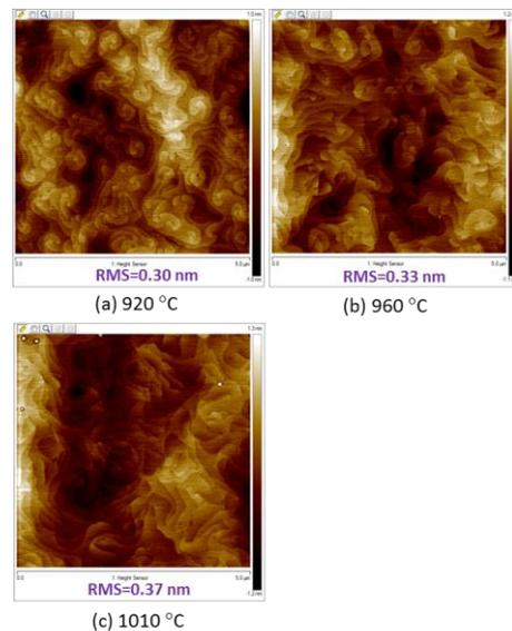
Fig. 4 5 μm x 5 μm AFM images of AlGa<sub>N</sub>/GaN heterostructures in N<sub>2</sub> ambient, (a) 920 °C, (b) 960 °C, (c) 1010 °C.
