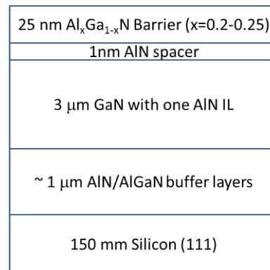
Fig. 1 Schematic of AlGa<sub>x</sub>N/GaN heterostructures on 150 mm (111) Si
