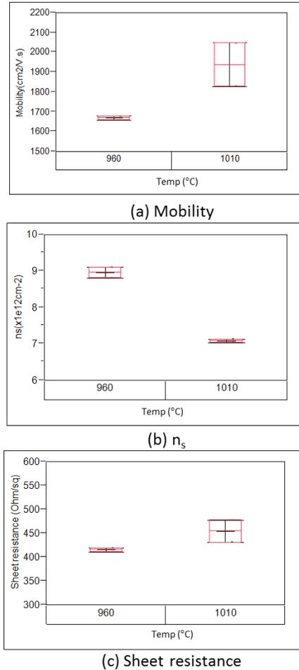
Fig. 3 Electrical properties of the AlGa<sub>N</sub>/GaN heterostructures in H<sub>2</sub> ambient at 960 °C and 1010 °C, (a) Mobility, (b) Sheet carrier concentration n<sub>s</sub>, (c) Sheet resistance.
