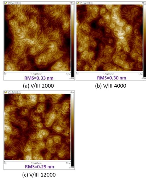
Fig. 6 5  $\mu m$  x 5  $\mu m$  AFM images of AlGaIn/GaN heterostructures with different V/III ratio, (a) V/III = 2000, (b) V/III = 4000, and (c) V/III = 12000 at 920 °C in  $N_2$  ambient.
