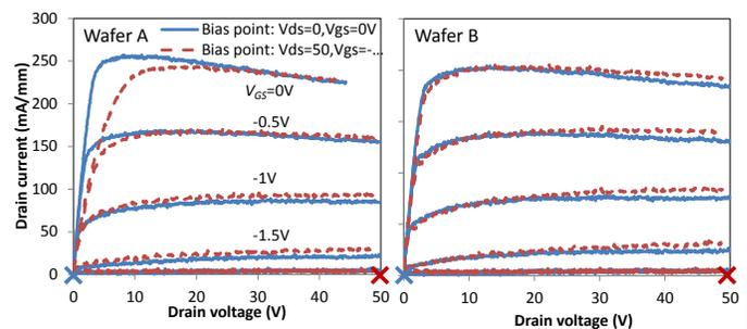
**Fig. 1:** Double pulse (DIVA) measurement of AlGaIn/GaN HEMTs from ON (blue lines  $V_{DS}=0, V_{GS}=0V$ ) and OFF (red dashed lines  $V_{DS}=50, V_{GS}=-3V$ ) quiescent bias points. Pulse durations 1 $\mu$ s/1ms,  $V_{GS}=0, -0.5 \dots -2.0V$ . Wafer A shows moderate current-collapse, whereas Wafer B is almost ideal.
