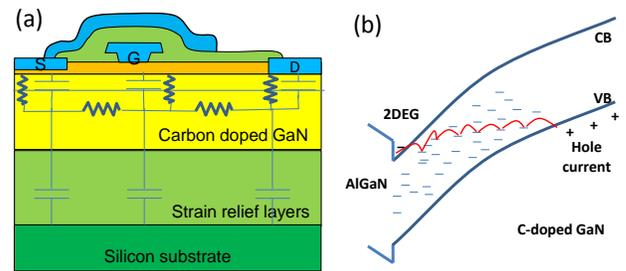
**Fig. 4:** (a) Schematic showing the vertical and lateral leakage and capacitive paths important in these GaN HEMTs. (b) Trap assisted tunneling process along a dislocation to inject holes from the 2DEG into the buffer during swept  $V_{SUB}$  measurement.
