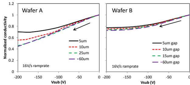
**Fig. 3:** Normalised sheet conductivity of ungated structures of varying gap size as  $V_{SUB}$  is swept from 0 to  $-200V$ .
