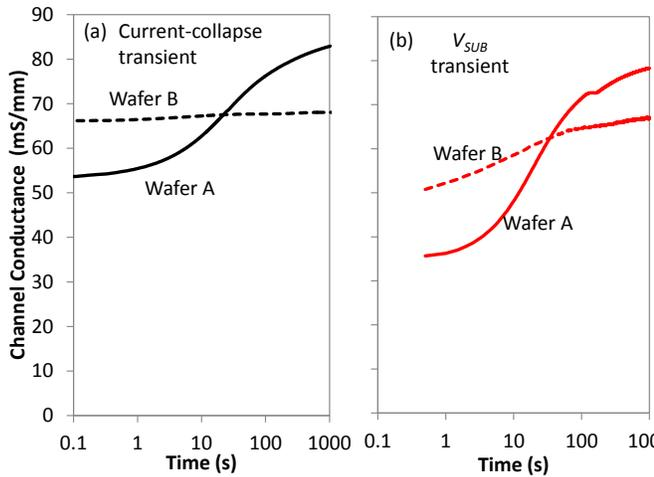
**Fig. 2:** Drain current transients (a) following step from OFF state ( $V_{DS}=50V$ ,  $V_{GS}=-3V$ ) to ON state ( $V_{DS}=1V$ ,  $V_{GS}=0V$ ), (b) following step from  $V_{SUB}=0$  to  $-200V$  with  $V_{DS}=1V$ . Similar time-constant and wafer dependence is observed indicating a common transient origin.
