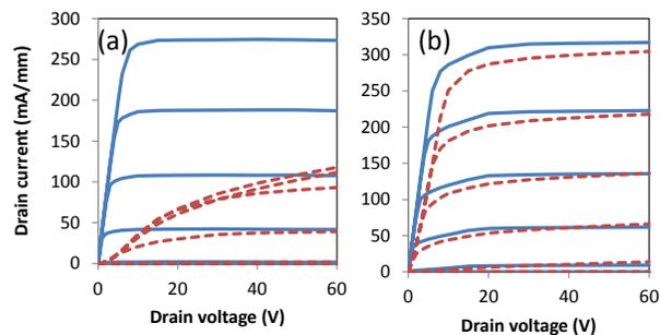
**Fig. 5:** Simulated double pulse (DIVA) measurements for the same conditions as in Fig. 1. (a) floating p-type buffer, whereas (b) has a P++ shorting region to the GaN buffer under the source and drain.
