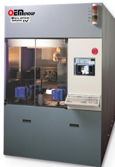
Fig. 1. MRC Eclipse Mark IV sputter tool equipped with plasma pre-clean chamber and three sputter chambers.
