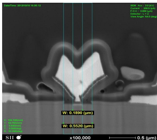
Figure 1: 0.18 \mu\text{m} T-gate profile on E-mode pHEMT
