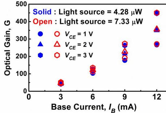
Fig. 4: The optical gain,  $G$ , of the HPT with different incident optical powers ( $P_{in} = 4.28$  and  $7.33 \mu\text{W}$ ) and biases.
