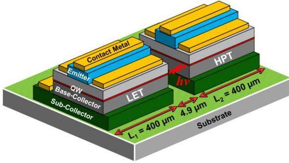
Fig. 1: Schematic device structure of two-section edge-emitting light-emitting transistor where one of them is operated as the light source (LET), and the other one is served as the photodetector (HPT).
