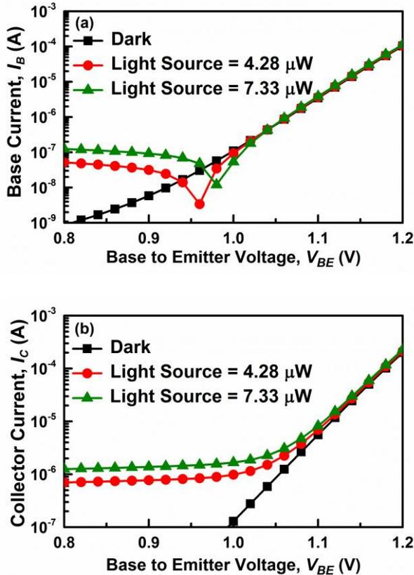
Fig. 2: (a) Base and (b) collector current of the HPT with illumination from LET (circles: 4.28  $\mu\text{W}$ ; triangles: 7.33  $\mu\text{W}$ ) and without illumination (squares).
