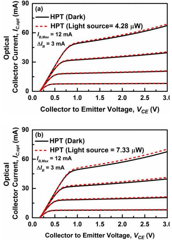
Fig. 3: The electrical characteristics of the HPT with incident optical power of (a) 4.28  $\mu\text{W}$  and (b) 7.33  $\mu\text{W}$  respectively.
