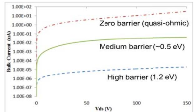
Figure 3. Bulk current for different effective barrier height in presence of deep traps.
