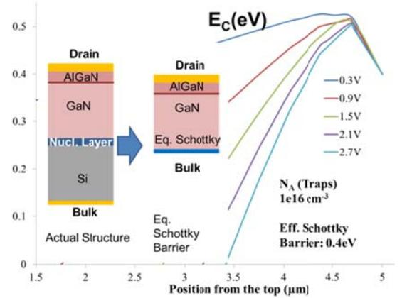
Figure 2. Effective Schottky barrier approach to simulating GaN/Si interface.  $E_c$  profiles show barrier height modulation at different voltages.
