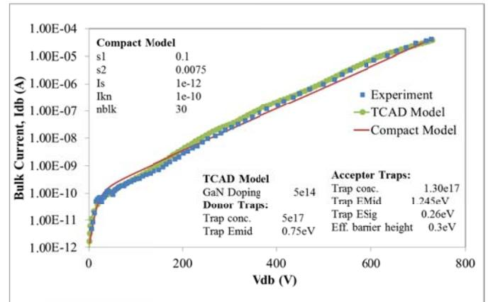
Figure 4. Fitting of the experimental I-Vs of the Figure 1 using the developed TCAD and compact model (CM)
