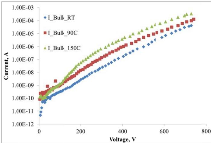
Figure 1. Experimental I-V characteristics measured at RT, 90C and 150C for two-terminal GaN on Si samples. At low voltages, the quasi-linear I-V slope corresponds to resistive current; at higher voltages the slope is proportional to  $\exp(V^{0.5})$  suggesting the field-dependent conductivity: Poole-Frenkel and/or barrier height modulation mechanisms. The I-V slope decrease with increasing temperature at higher voltages:  $I \sim \exp(kT^{-1})$  also agrees with the suggested mechanisms.
