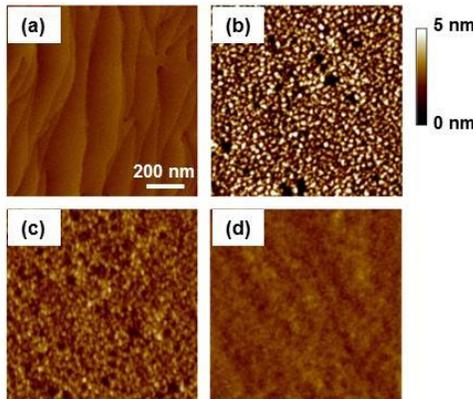
Fig. 1 AFM images of GaN surface etched by  $\text{BCl}_3$  etching process : (a) as-grown, (b) bias power 1.5 W, (c) bias power 3 W, (d) bias power 10 W.
