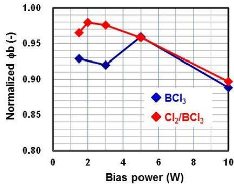
Fig. 5 Comparison of the normalized  $\phi_b$  obtained from  $\text{BCl}_3$  etching process and  $\text{Cl}_2/\text{BCl}_3$  etching process.
