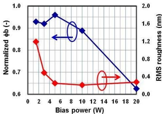
Fig. 2 Etching bias power dependence on the normalized  $\phi_b$  and RMS roughness obtained from  $\text{BCl}_3$  etching process.
