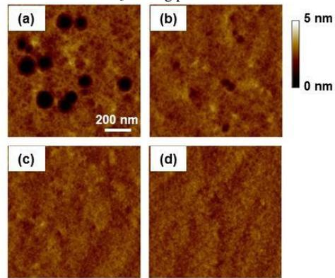
Fig. 3 AFM images of GaN surface etched by  $\text{Cl}_2/\text{BCl}_3$  etching process : (a) bias power 1.5 W, (b) bias power 2 W, (c) bias power 3 W, (d) bias power 10 W.
