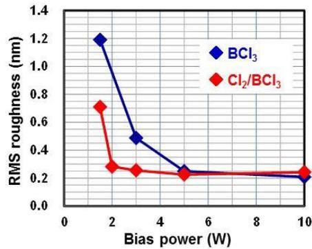
Fig. 4 Comparison of RMS roughness obtained from  $\text{BCl}_3$  etching process and  $\text{Cl}_2/\text{BCl}_3$  etching process.
