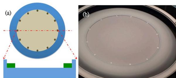
Fig. 2. (a) Illustration of the sapphire pits on susceptor; (b) The picture for the sapphire pits distribution on the susceptor.
