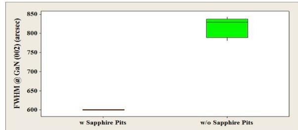
Fig. 5. The FWHM @ GaN(002) for the sample with and without sapphire pits.
