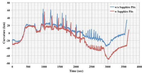
Fig.3. The in-situ curvature measurement for the samples growth with sapphire pits and without sapphire pits”.
