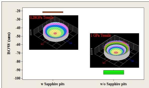
Fig. 4. The stress measurement result exhibited for the sample with and without using sapphire pits.
