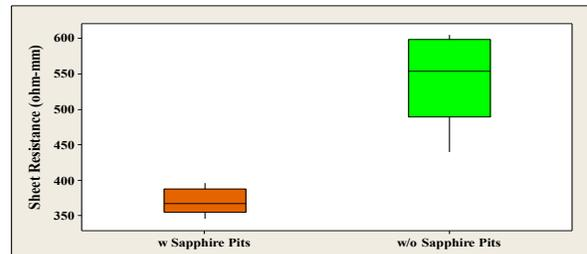
Fig.6. The sheet resistance for the samples with and without sapphire pits.
