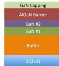
Fig.1. The epitaxial structure for all samples.
