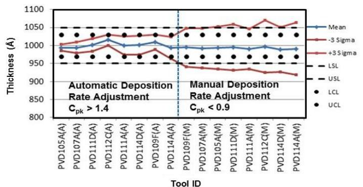
**Figure 3. Results of implementation of automatic deposition rate adjustment for all sputter tools.**
