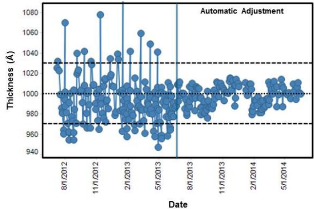
**Figure 2. Thickness of Ti film deposition before and after the application of automatic deposition rate adjustment.**
