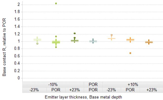
**Figure 3:** Base contact resistance for each emitter layer thickness and base metal depth combination.
