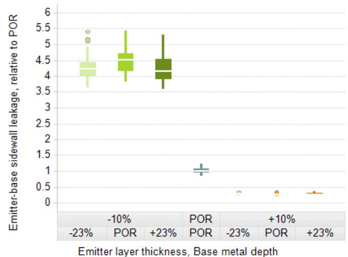
**Figure 2:** Emitter-base leakage for each emitter layer and base metal depth combination.
