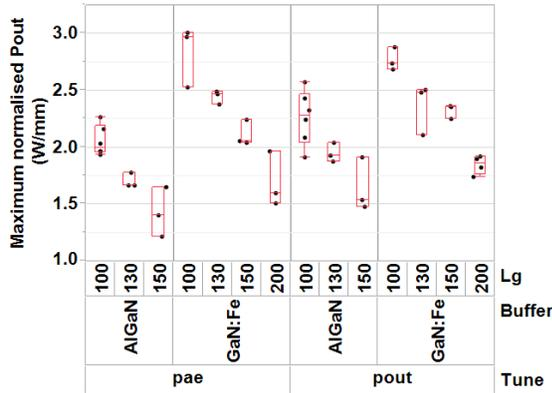
Figure 2 – Results of load-pull measurements of  $8 \times 100 \mu\text{m}$  transistors at 10 GHz
