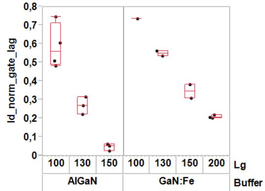
Figure 3 - Normalized drain current drop caused by gate lag
