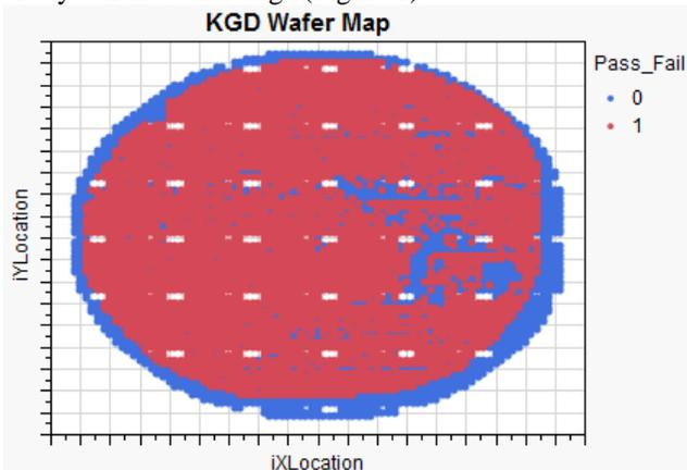
Figure 1. KGD map of a typical low-yield PHEMT wafer; red is passed die, blue is failed die.
