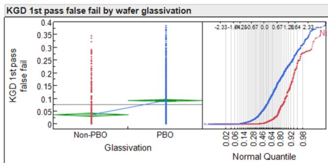
Figure 1. KGD first pass false fail rate for wafers with and without PBO coating. Quantile plot also shows significant difference between the two types of wafers.
