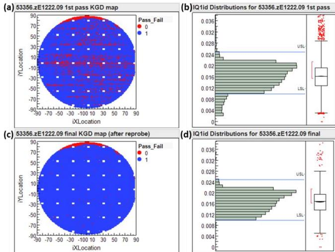
Figure 2. (a) KGD first pass map (red – fail, blue – pass) and (c) final map after retest. (b) and (d) are distribution of IQ1id, a test parameter sensitive to probe touch quality.
