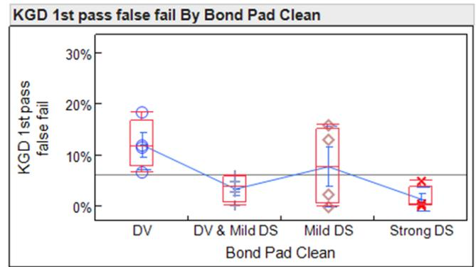
Figure 3. KGD first pass false fail rates for wafers etched only in PBO developer (DV), wafers etched in developer followed by mild plasma etch (DV & Mild DS); wafer plasma etched only at low power (Mild DS); wafer plasma etch only at high power (Strong DS).
