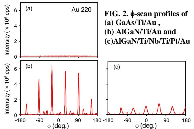
FIG. 2.  $\phi$ -scan profiles of (a) GaAs/Ti/Au, (b) AlGaIn/Ti/Au and (c) AlGaIn/Ti/Nb/Ti/Pt/Au
