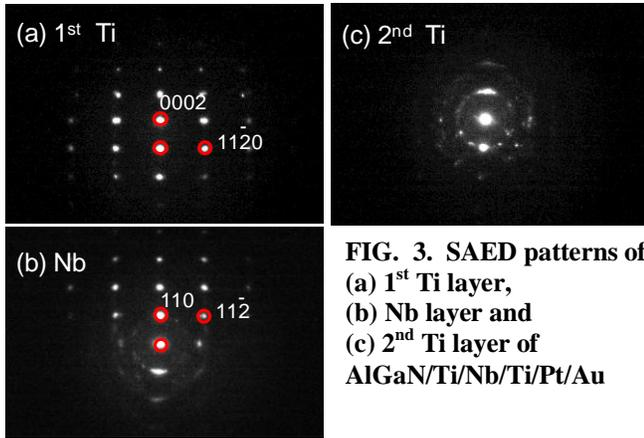
**FIG. 3. SAED patterns of (a) 1<sup>st</sup> Ti layer, (b) Nb layer and (c) 2<sup>nd</sup> Ti layer of AlGaIn/Ti/Nb/Ti/Pt/Au**
