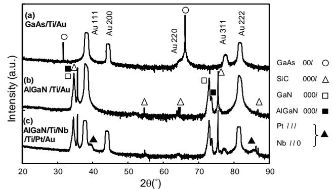
FIG. 1.  $2\theta$ - $\omega$  scan profiles of (a) GaAs/Ti/Au, (b) AlGaIn/Ti/Au and (c) AlGaIn/Ti/Nb/Ti/Pt/Au
