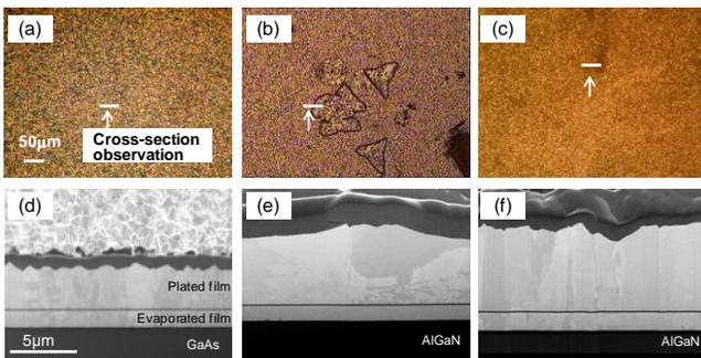
**FIG. 4. Surface morphologies of (a) GaAs/Ti/Au, (b) AlGaIn/Ti/Au and (c) AlGaIn/Ti/Nb/Ti/Pt/Au. Cross-section SEM images of (d) GaAs/Ti/Au, (e) AlGaIn/Ti/Au and (f) AlGaIn/Ti/Nb/Ti/Pt/Au**
