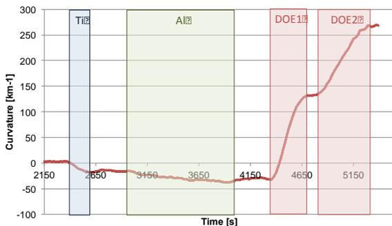
FIGURE 2: Evolution of stress in a Ti/Al / Ni coating
