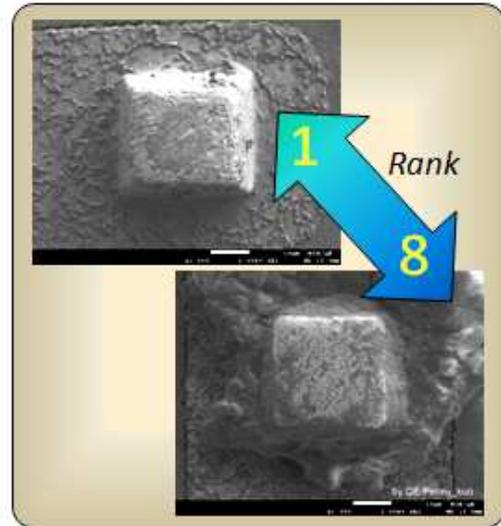
Fig.4 Ranking and Numeralization for the particle on the probe tip.
