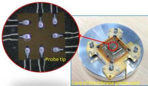
Fig.2 Probe tip and membrane probe card core
