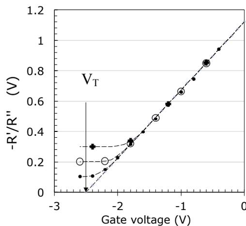
**Fig.5.** Standard  $I_{DS}/\sqrt{g_m}$  ratio method applied to the data of Fig.3. The curvature of the curve renders the extraction of a threshold voltage difficult. The intercept of the dashed curve is more than 150mV apart from the true threshold voltage.
