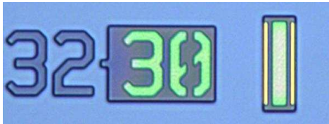
Figure 2. The new CD structure is shown in the far right. The new structure closely matches the product device topography and feature size.
