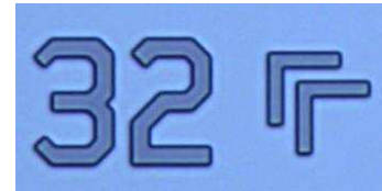
Figure 1. The standard artifact used to measure in-line critical dimensions, here shown for layer 32.
