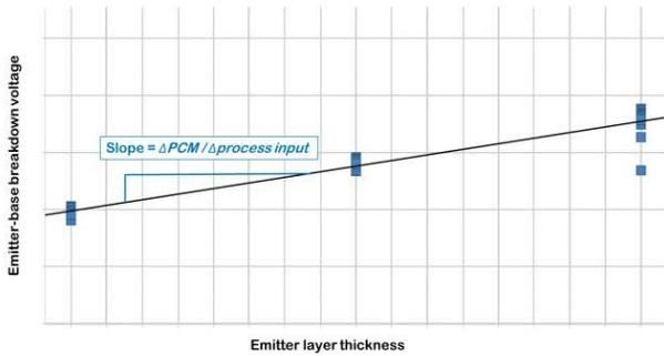
**Figure 5:** Example of how emitter-base breakdown changed with emitter layer thickness in the process margin study.
