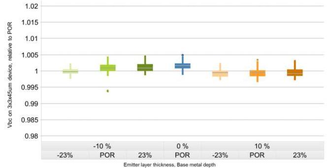
**Figure 4:** Base collector turn on voltage over process margin variants.
