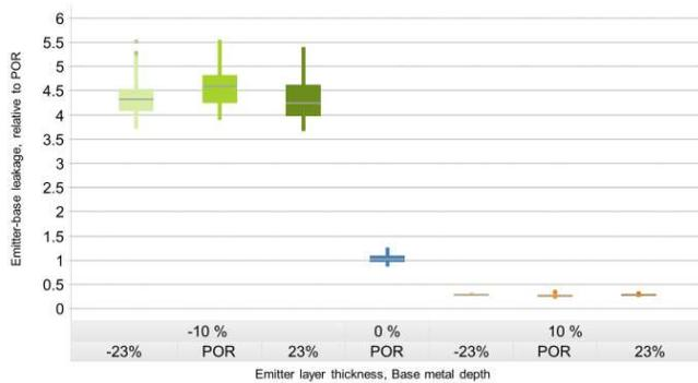
**Figure 2:** Emitter-base leakage for each emitter layer and base metal depth combination.
