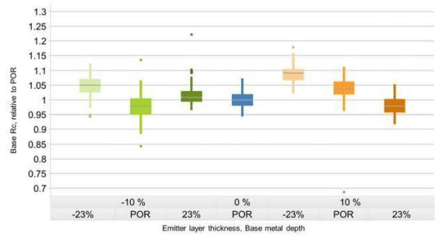
**Figure 3:** Base contact resistance for each emitter layer thickness and base metal depth combination. Note that for emitter layer thickness POR+10%,  $R_c$  Base appears to be correlated to base metal depth, but at POR-10%, it does not.
