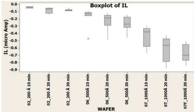
Figure 6: Box plot of the gate drain leakage current measured at -7 V.
