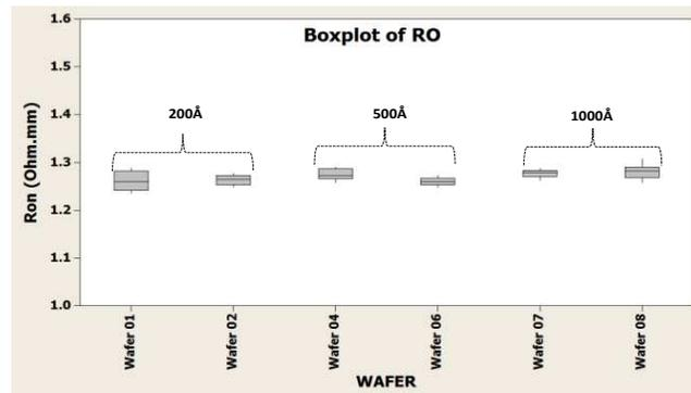
Figure 3: On resistances measured at the drain source linear zone at a gate bias of 0V. Measured before anneal testing.
