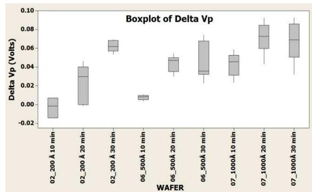
Figure 4: Boxplot of delta Vp for varying Pt thickness after 10, 20 and 30 minutes of annealing at 300°C.
