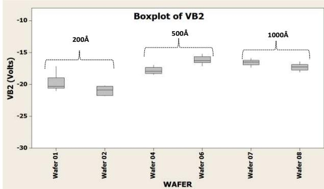
Figure 2: Gate drain breakdown voltages (Vb2) measured at 1mA/mm current before anneal testing.
