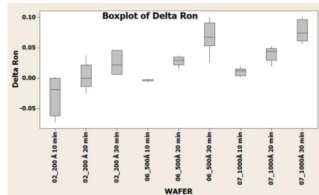
Figure 5: Box plot of delta on resistances for varying platinum thicknesses after each anneal step.
