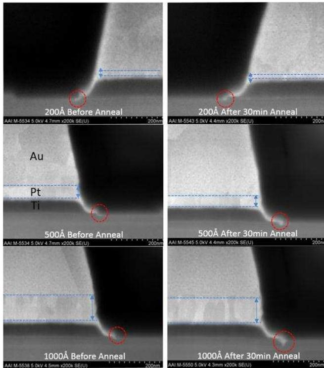
Figure 7: FIB cross-sections of the gates before and after the total anneal time of 30 minutes at 300°C.
