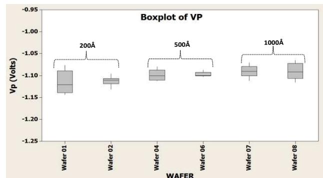
Figure 1: Pinch off voltages ( $V_p$ ) measured at 2.5% of  $I_{dss}$ . The above values are taken before any anneal testing.
