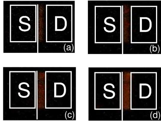
Fig. 3 Electroluminescence profile of the device with O<sub>2</sub> plasma treatment. (a)  $V_{ds} = 800$  V, (b)  $V_{ds} = 1200$  V, (c)  $V_{ds} = 1400$  V, and (d)  $V_{ds} = 1600$  V.
