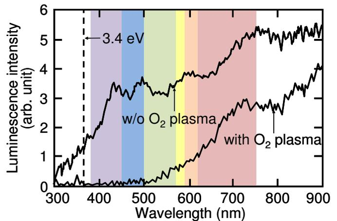
Fig. 4 Measured EL intensity as a function of photon wavelength. Visible spectrum range from 380 to 750 nm is covered for device without O<sub>2</sub> plasma treatment.
