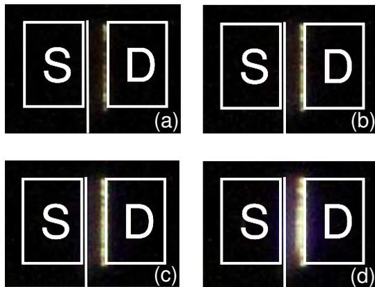
Fig. 2 Electroluminescence profile of the device without O<sub>2</sub> plasma treatment (reference A). (a)  $V_{ds} = 1000$  V, (b)  $V_{ds} = 1100$  V, (c)  $V_{ds} = 1200$  V, and (d)  $V_{ds} = 1400$  V.
