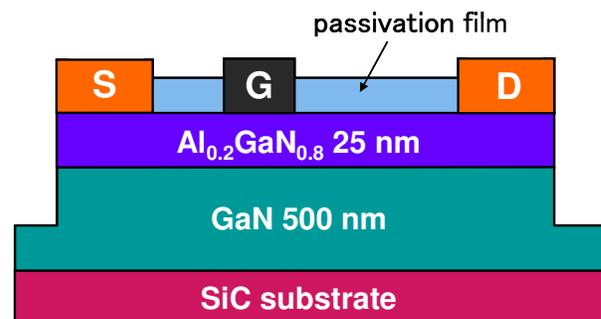
Fig.1 Cross-section of fabricated AlGa<sub>N</sub>/Ga<sub>N</sub> HEMT.
