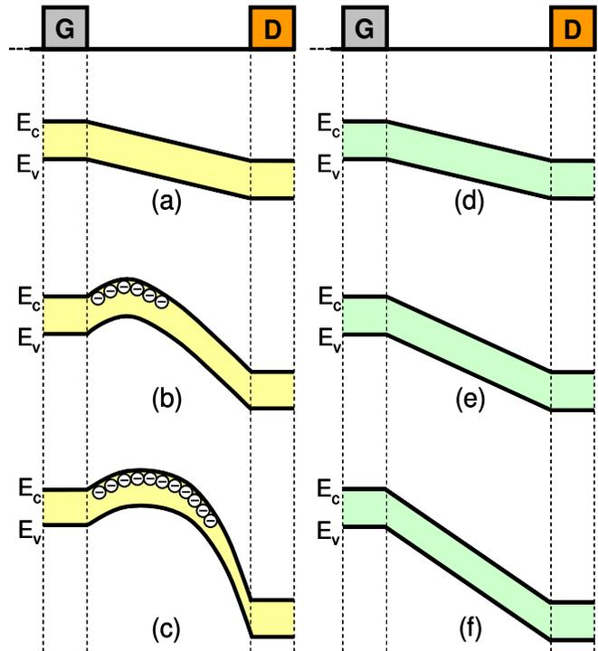
Fig. 5 Schematic drawings of potential distribution between gate and drain for devices under drain bias from low to high values: device with high density of surface trap states (a), (b), and (c), and device with low density of trap states (d), (e), and (f).
