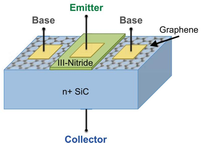
Figure 1. Schematic diagram of a III-nitride/graphene/SiC vertical transport hot electron transistor.
