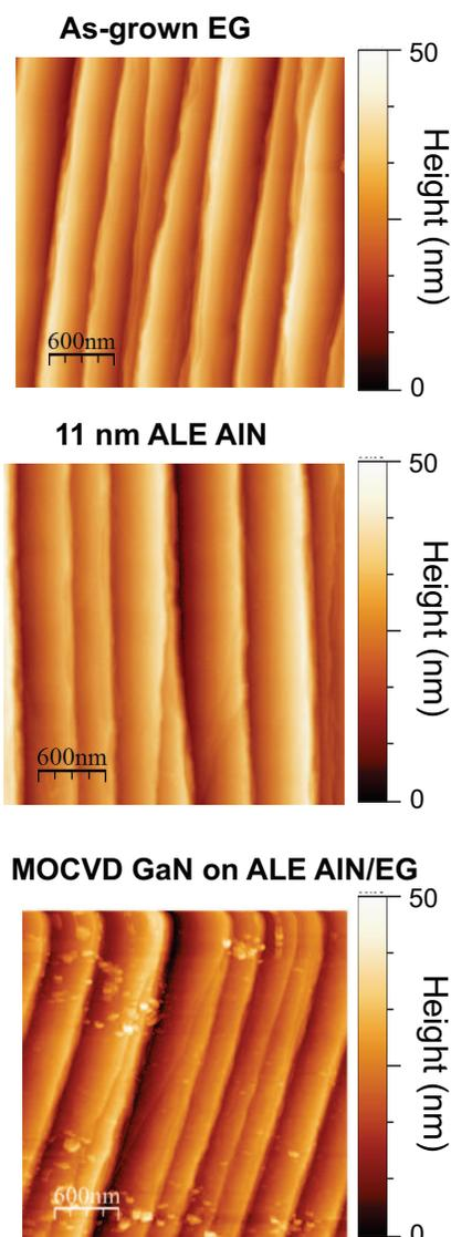
Figure 2. AFM images of As-grown EG surface, after growth of 11 nm of ALE AlN, then after growth of MOCVD GaN on the ALE AlN/EG [5].
