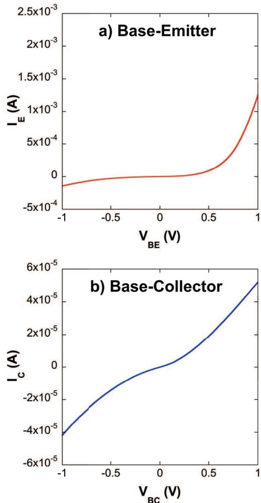
Figure 4. I-V characteristics for a) base-emitter (graphene-III-nitride) and b) base-collector (graphene-SiC).
