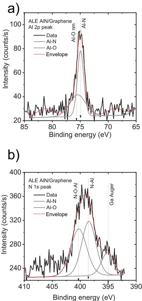
Figure 3. High resolution XPS spectra of Al 2p and N 1s peaks are shown in Fig. Fitting In 3d and N 1s peaks indicates the presence of Al-O besides Al-N. Ga Auger peak is due to ~1 nm GaN cap layer
