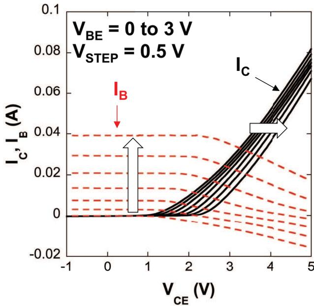
Figure 5. Three terminal measurement of the III-nitride/graphene/SiC device.
