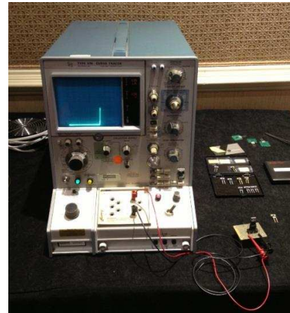
Figure 1: Curve tracer picture showing breakdown on a GaN p-n diode. The horizontal axis is 200V/division.
