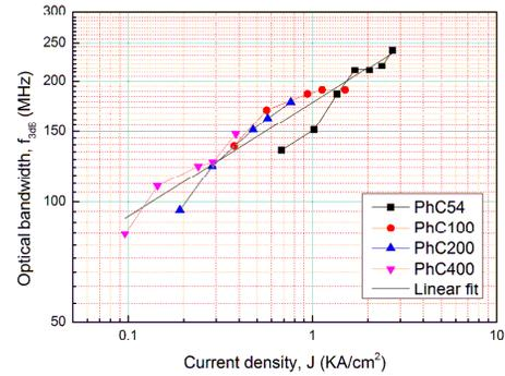
Figure 6: The modulation bandwidth as a function of the injected current density of PhCLEDs.
