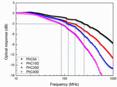
Figure 4: Frequency response of different PhCLEDs at a 50 mA injection current.
