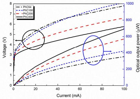
Figure 2: Optical output and electrical property of different PhCLEDs.
