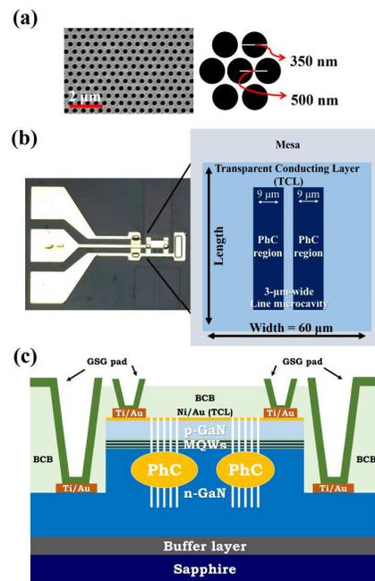
Figure 1: (a) SEM of the design PhCs. (b) Layout of the light-emitting area and PhC region. Left inset is the OM image of PhC54. (c) Cross-sectional structure of PhCLED.
