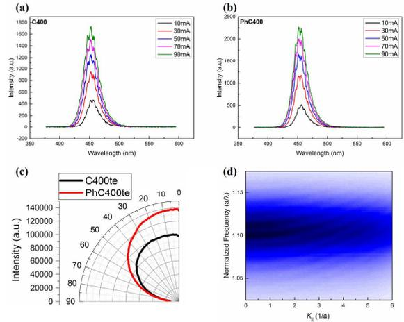
Figure 3: Optical properties of the CLED and the PhCLED. Electroluminescence (EL) spectra of the (a) C400 and (b) PhC400. (c) Angular-resolved profiles of the C400 and PhC400. (d) Measured photonic band of the PhC400.
