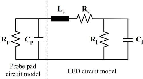
Figure 5: Small-signal equivalent model of the LEDs with RF probe pads.
