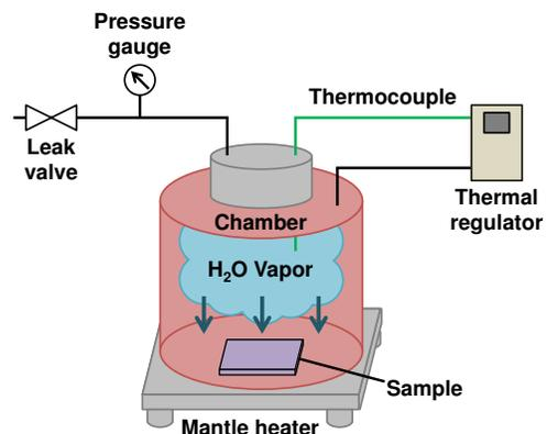
Fig. 1 Schematic illustration of high pressure water vapor annealing (HPWVA) experimental set-up.
