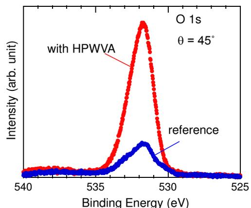
Fig. 6 O 1s XPS spectra of reference and HPWV-annealed (with HPWVA at 400 °C) samples taken at escape angle  $\theta = 45^\circ$ .
