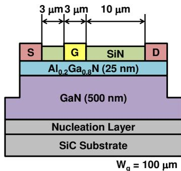
Fig. 2 Schematic cross-sectional illustration of AlGaIn/GaN HEMT used in this study.
