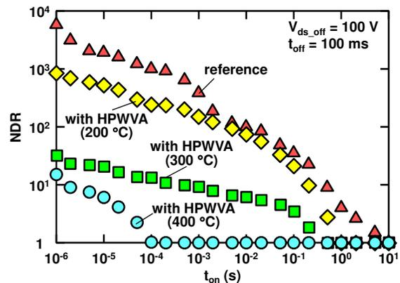
Fig. 4 Normalized dynamic  $R_{on}$  (NDR) dependence on on-time  $t_{on}$  of reference and HPWV-annealed devices.
