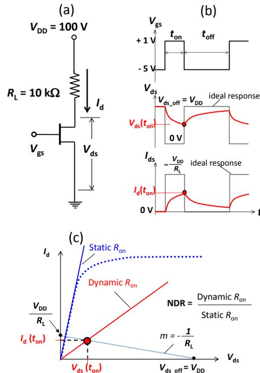
Fig. 3 Schematic illustration of (a) electrical circuit used in current collapse evaluation, (b) current and voltage waveforms, (c) load-line and dynamic  $R_{on}$  graphical definition.
