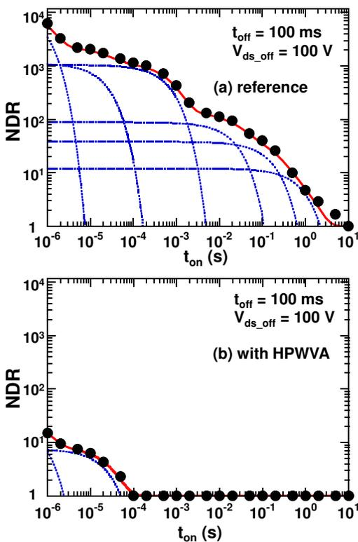
Fig. 5 Measured (solid data points) and calculated (solid curves) normalized dynamic  $R_{on}$  (NDR) dependence on  $t_{on}$  of (a) reference and (b) HPWV-annealed at 400 °C devices. Dashed curves represent extracted exponential terms.
