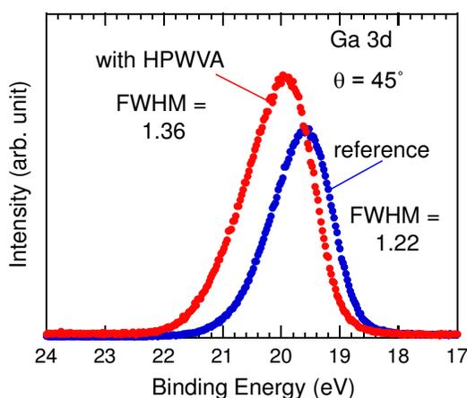
Fig. 7 Ga 3d XPS spectra of reference and HPWV-annealed (with HPWVA at 400 °C) samples taken at escape angle  $\theta = 45^\circ$ .
