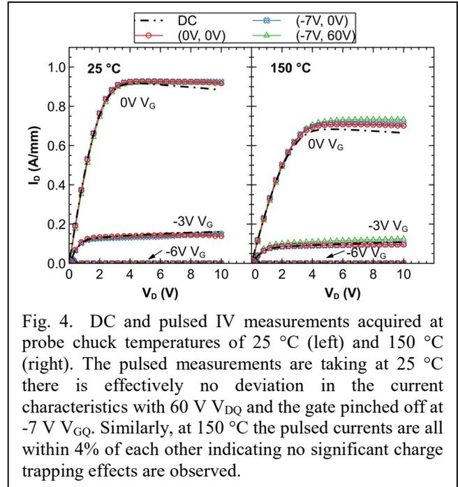
Fig. 4. DC and pulsed IV measurements acquired at probe chuck temperatures of 25  $^\circ\text{C}$  (left) and 150  $^\circ\text{C}$  (right). The pulsed measurements are taking at 25  $^\circ\text{C}$  there is effectively no deviation in the current characteristics with 60 V  $V_{DQ}$  and the gate pinched off at -7 V  $V_{GQ}$ . Similarly, at 150  $^\circ\text{C}$  the pulsed currents are all within 4% of each other indicating no significant charge trapping effects are observed.
