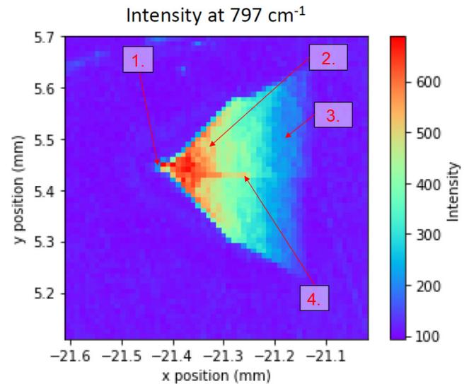
Figure 3. Micro Raman intensity of 797  $\text{cm}^{-1}$  line that corresponds to 3C-SiC.
