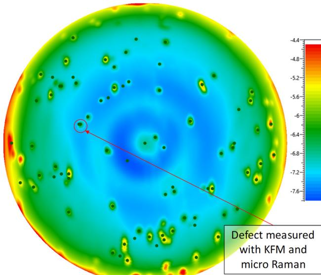
Figure 1. The QUAD map of electrically active defects in epitaxial 4H-SiC wafer.
