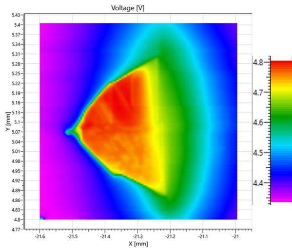
Figure 2a. Work function of a triangular defect measured with the KFM showing as much as 4.8eV for 3C-SiC within a defect decreasing to 4.3eV for 4H-SiC outside the defect.
