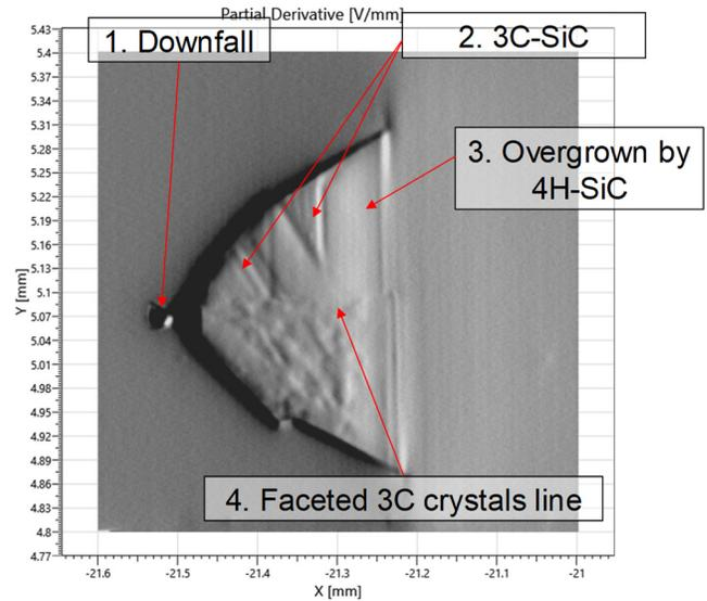
Figure 2b. 4 elements identified on the differential KFM map: downfall, 3C-SiC, faceted 3C crystals line, and the base with 3 C-SiC overgrown by 4H-SiC.
