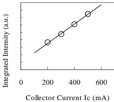
Figure 2 Collector current dependence of integrated EL intensity
