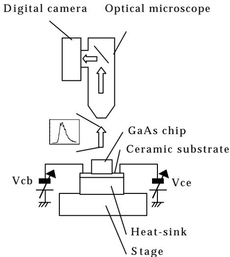
Figure 6 Setup of the measurement system
