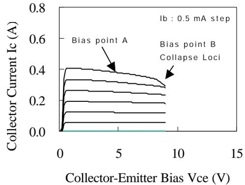
Figure 7-a  $I_c$ - $V_{ce}$  characteristics of sample I
