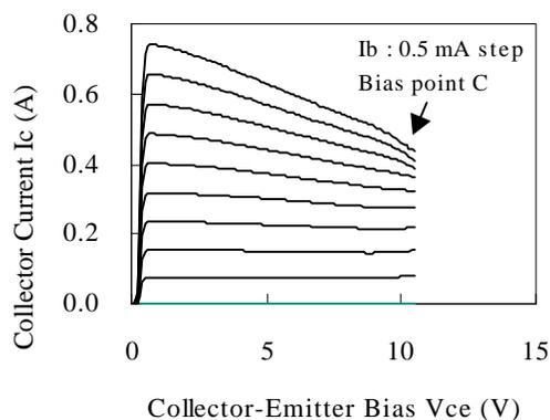
Figure 8-a  $I_c$ - $V_{ce}$  characteristics of sample II
