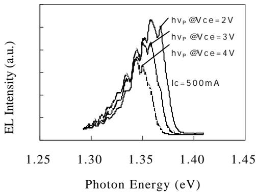
Figure 3 EL spectra for  $V_{ce}$  from 2 V to 4 V (@  $I_c = 500$  mA)
