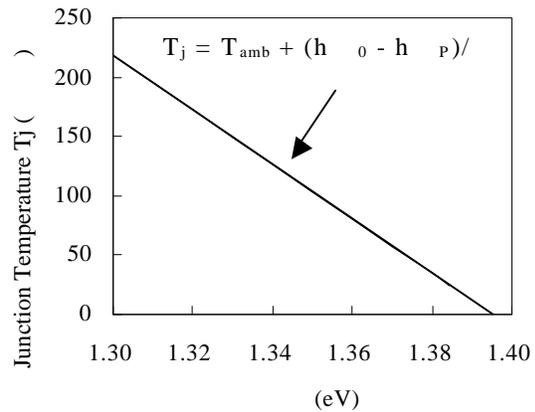
Figure 5 Junction temperature  $T_j$  as a function of  $h\nu_p$
