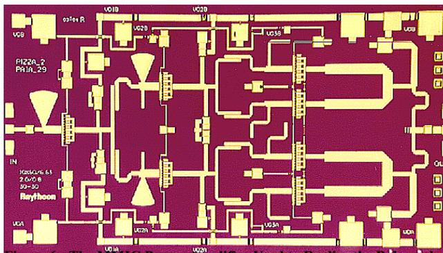
**Figure 6:** The MMIC Power Amplifier Used to Realize the Balanced RF Output Stage. This is a 27-32 GHz Device With a Nominal 17 dB of Gain and a Saturated Power Output of +30 dBm.
