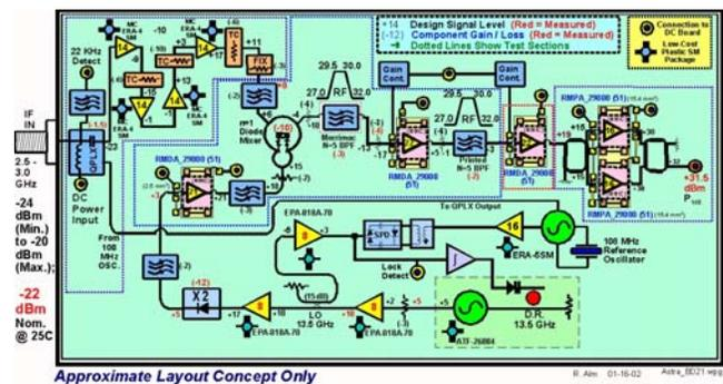
**Figure 2:** System Block Diagram Showing the Basic Functions of the Up-Converter Transmit Module.
