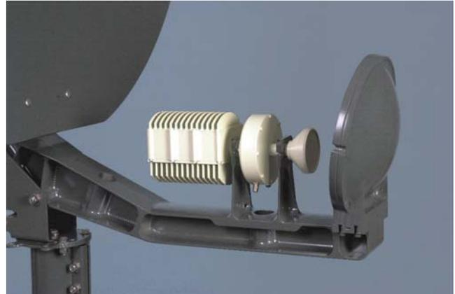
**Figure 1:** The Key Elements of the Outdoor Unit. The Sub-Reflector (Right) Faces the Feed (horn); the LNB is the Round Element, and the Transmit Module (with Heat Dissipation Fins) is Mounted Behind the LNB and Above the Boom.
