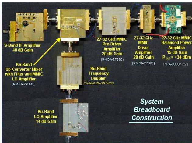
**Figure 10:** The Major Functions of the Block Diagram Shown in Figure 2 Are Built, Tested and Evaluated at the System Level.
