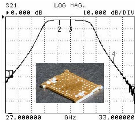
**Figure 7:** The Sharp Cutoff Bandpass Filter Realized Using Merrimac Industries' Multi-Mix® Technology. This Component Enabled Single-Up Conversion Critical to the Low-Cost Approach.
