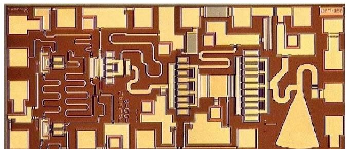
**Figure 5:** The MMIC Amplifier Used as the RF Pre-Driver, the RF Driver and the LO Amplifier at 29.5-30 GHz and at 27 GHz Respectively. This is a Wideband 20-42 GHz Device With a Nominal 20 dB of Gain and a Saturated Power Output of +22 dBm.
