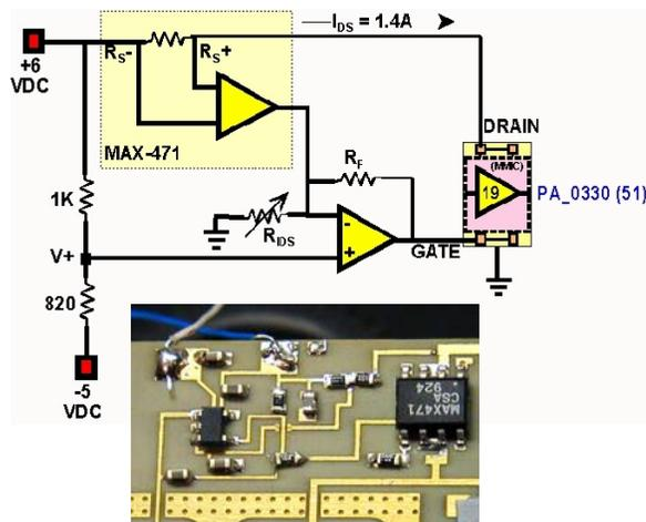
**Figure 8:** Active Bias Circuits Make MMIC Devices Insensitive to Pinchoff Voltage Variation and Can Also Help to Compensate for Gain Variation with Temperature.
