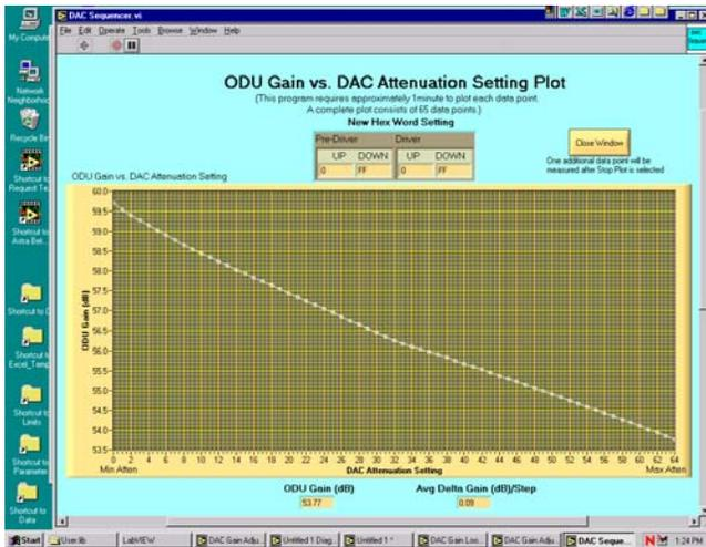
**Figure 9:** The Microprocessor Controlled MMIC Gate Bias Adjustment Gave the Module an Overall Gain Adjustment Range of about 7 dB.
