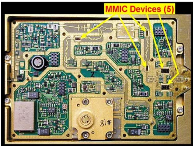
**Figure 3:** A Single Soft-Substrate Contains All RF Components. Prior to Bolting the RF Baseplate into the Module, Nothing Interferes with Automatic Assembly Tools in Manufacturing.
