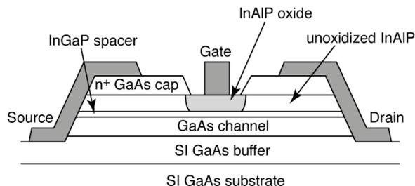
Figure 2. Cross-section of InAlP-oxide based MOSFET.
