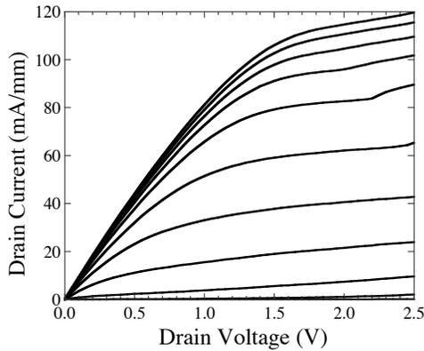
Figure 5. Common-source characteristics of 1  $\mu\text{m}$  gate length, 100  $\mu\text{m}$  gate width depletion-mode MOSFET.
