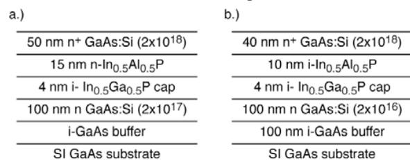
Figure 1. Cross-sectional diagram of heterostructures for (a) depletion-mode and (b) enhancement-mode GaAs-channel MOSFETs.
