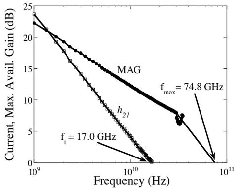
Figure 8. Microwave performance of typical 1  $\mu\text{m}$  gate length depletion mode device.
