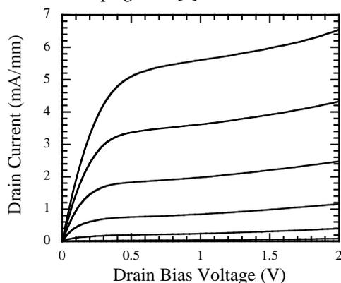
Figure 3. Common-source characteristics of enhancement-mode MOSFET with  $2 \mu\text{m}$  gate. Gate voltage stepped from  $-0.2 \text{ V}$  to  $0.5 \text{ V}$  in  $0.1 \text{ V}$  steps.
