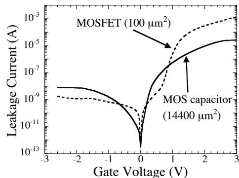
Figure 7. Leakage current of MOSFET gate and MOS capacitor test structure. MOSFET exhibits higher leakage due to gate contact with mesa edge, while MOS capacitor reflects intrinsic oxide leakage.
