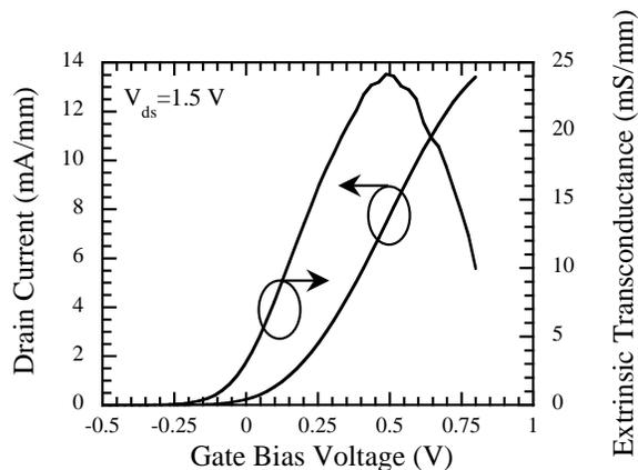
Figure 4. Drain current and extrinsic transconductance as a function of gate voltage for  $2 \mu\text{m}$  gate length enhancement-mode MOSFET.
