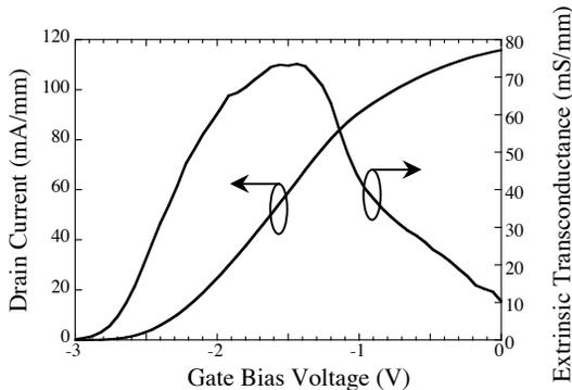
Figure 6. Drain current and transconductance vs. gate voltage for 1  $\mu\text{m}$  gate length depletion-mode MOSFET.
