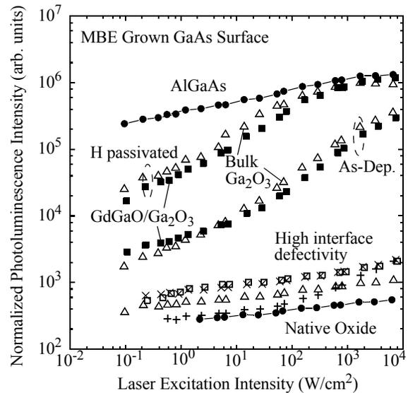
Fig. 3 Normalized GaAs photoluminescence intensity as a function of excitation intensity for AlGaAs (solid circles),  $\text{Ga}_2\text{O}_3$  (open triangles), GdGaO/ $\text{Ga}_2\text{O}_3$  (solid squares), high interface defectivity films, and native oxide (solid circles) on GaAs. All materials are deposited on MBE grown surfaces under UHV conditions (except for native oxide).
