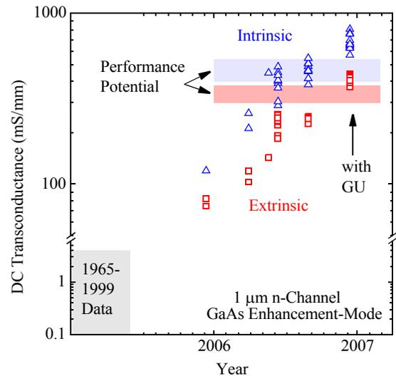
Fig. 1 Evolution of DC transconductance of GaAs based MOSFETs. (GU: Glasgow University)
