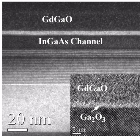
Fig. 2 Dark field TEM micrograph of a typical MOSFET structure with an InGaAs channel. The inset shows a high resolution TEM micrograph of the oxide/semiconductor interface.
