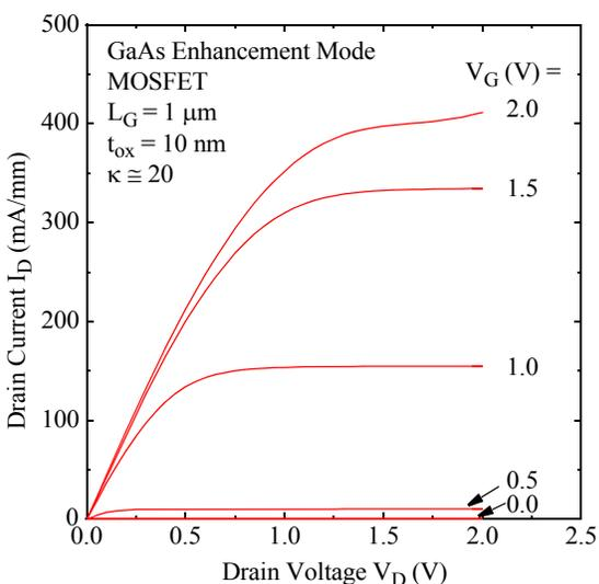
Fig. 5 Output characteristics of a 1  $\mu\text{m}$  GaAs MOSFET.
