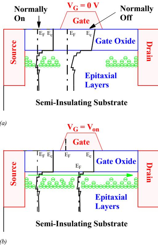
Fig. 4 Implant free (flatband) MOSFET in off-state (a) and on-state (b).
