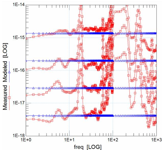
Figure 3. Extreme case of non-1/f noise behavior (GaAs MESFET device, noise spectral density is frequency-normalized, in units of A<sup>2</sup>). The extracted frequency exponent value is in this case 0.73.
