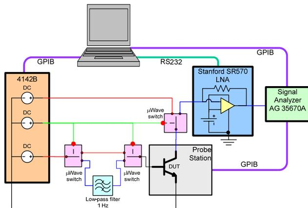
Figure 1. Diagram of the 1/f noise test setup.
