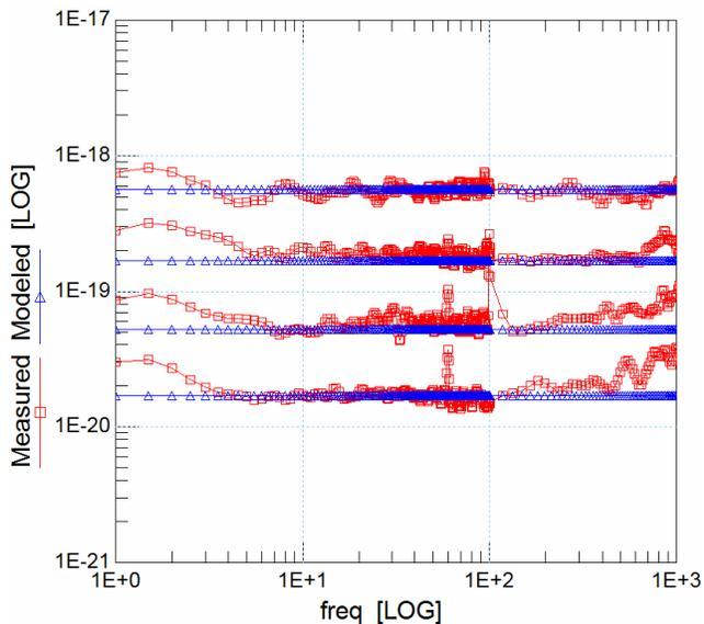
Figure 4. Close to ideal 1/f noise behavior (Si bipolar device, noise spectral density is frequency-normalized, in units of A<sup>2</sup>). The extracted frequency exponent value is in this case 1.13.
