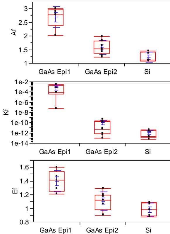
Figure 6. Comparison of extracted Flicker noise parameters for various device selections.
