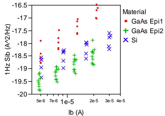
Figure 5. Comparison of fitted 1 Hz noise data versus base current for various device selections.
