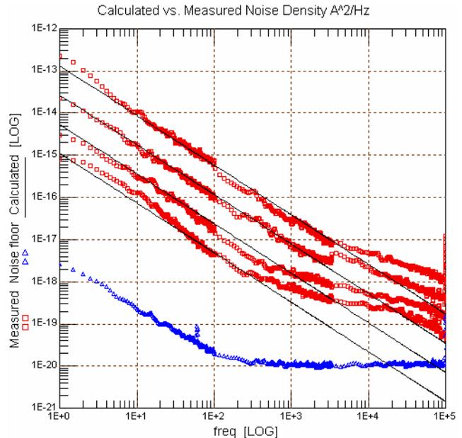
Figure 2. Example of measured 1/f noise spectral density at HBT collector (GaAs) versus the worst system noise floor.
