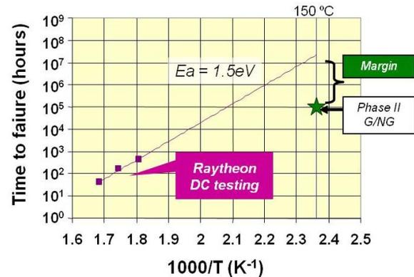
Figure 2. MTTF projection for Raytheon devices at the end of Phase II, with a MTTF of  $> 10^6$  hours at a junction temperature of  $150^\circ\text{C}$  based upon tests at 280, 300 and  $320^\circ\text{C}$ .
