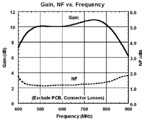
Figure 10: Gain and NF characteristics of DTV LNA
