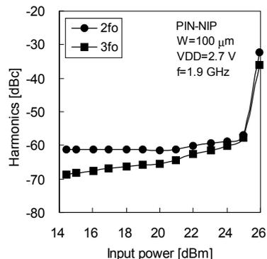
Figure 3: Harmonics characteristics of the ESD protection device
