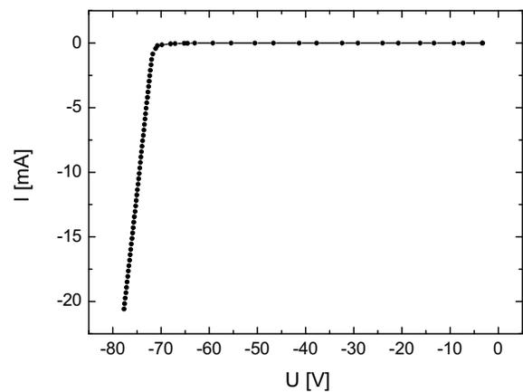
Fig. 3: Reverse characteristic of a 20-finger power Schottky diode showing its high-current blocking capability at voltages higher than 70 V.
