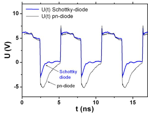
Fig. 4: Time-domain measurements giving a recovery time of 590 ps (extracted 12.1 ps for intrinsic diode) for 20 finger power Schottky diode in comparison with similar pn-diode (recovery time of 2.2 ns, extracted 45 ps for intrinsic diode) obtained with square-wave input signal of 180 MHz,  $V_{pp} = 13$  V.
