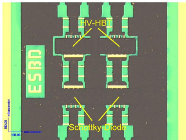
Fig. 1 Viewgraph of integrated HV-HBTs and Schottky diodes prepared for flip-chip mounting.
