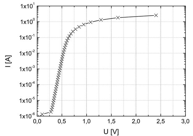
Fig. 2: Forward characteristic of a 20-finger power Schottky diode showing its high-current driving capability.
