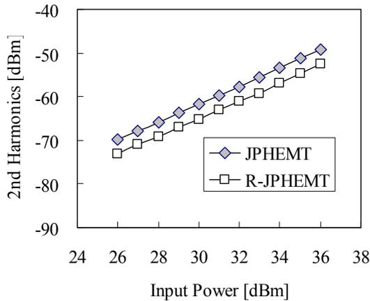
Fig.4 The relation of the 2<sup>nd</sup> harmonics to an input power@900MHz
