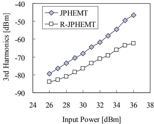
Fig.5 The relation of the 3<sup>rd</sup> harmonics to an input power@900MHz
