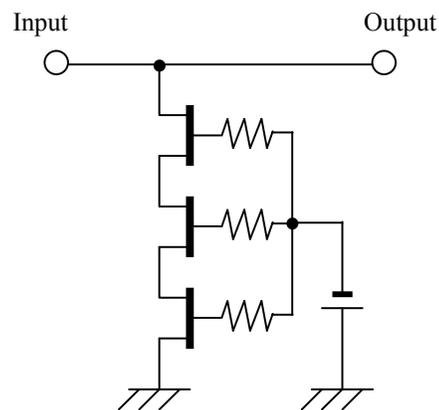
Fig.3 Schematic of distortion measurement of off-state device
