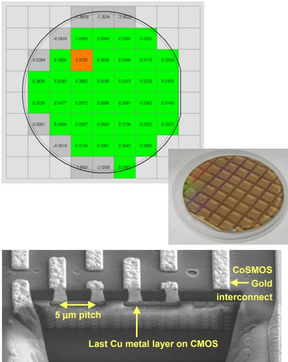
Figure 7. Wafer map showing the unit resistance in ohms of a 1000 unit long heterogeneous interconnect via chain with a 5 $\mu$ m pitch and 1.0x1.0 $\mu$ m<sup>2</sup> via size. Fully processed wafer and a cross sectional SEM of the via chain are also shown.
