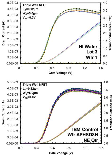
Figure 4. Transfer IV characteristics and associated transconductance, gm, from a 1.5V thin-oxide, triple-well NFET (LG=120nm, WG=5.0μm) bias at a VDS=1.5V and VBS=0.0V. A sparse sampling of 10 devices from a single HI wafer (top) and 22 devices from a quarter of the IBM control CMOS wafer (bottom) are shown.
