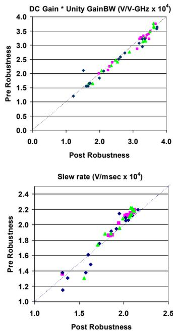
Figure 8. HI differential amplifier slew rate (bottom) and DC gain x unity gain bandwidth (top) comparison before and after 100 of -55 $^{\circ}$ C to +85 $^{\circ}$ C temperature cycles, indicating that the HI ICs are robust.
