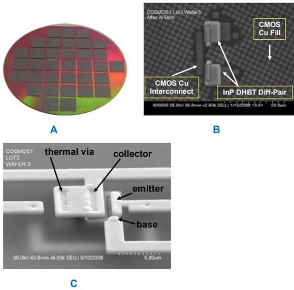
Figure 3. a) A photograph of an die bonded wafer at step E of Figure 2, b) an SEM micrograph HI integrated HBT before final interconnection, and c) an SEM micrograph of an HBT at the end of the process.
