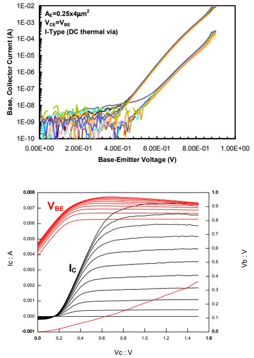
Figure 5. DC characteristics of an  $A_E=0.25 \times 4.0 \mu\text{m}^2$  InP DHBT bonded onto CMOS: (top) forward Gummel with DC current gain ( $\beta_f$ ) >30 while being driven at an  $I_C=10\text{mA}/\mu\text{m}^2$  and a  $V_{CE}=V_{BE}$ ; (bottom) common emitter IV and corresponding  $V_{BE}$  with  $I_B=0$  to  $200\mu\text{A}$  in  $20\mu\text{A}$  steps.
