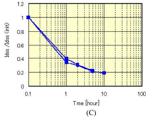
**Figure 5** Accelerated test of the device on various off-angle wafers, (A) 0.06° (B) 0.11° (C) 0.47°.
