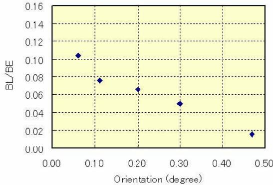
**Figure 4** The BL and BE ratio of Photo luminescence dependency on SiC wafer orientation angle
