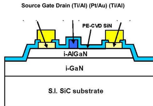
Figure 1 Cross-section of device structure.
