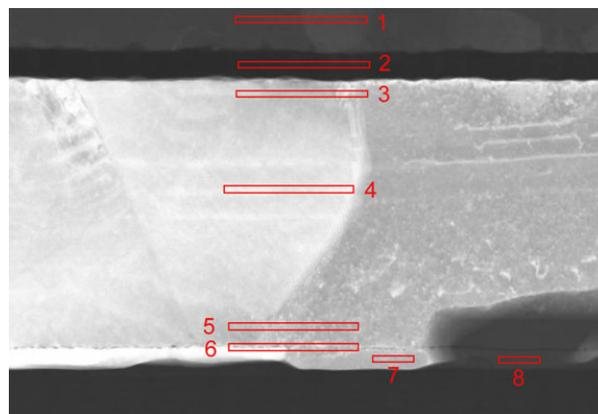
**Figure 2 STEM image of Cu Metal 1 on Ohmic**
