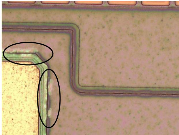
**Figure 1 Exposed Cu attacked in pre-clean solution.**
