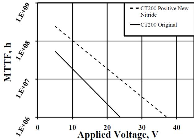
Figure I: MTTF as a function of a constant input applied voltage
