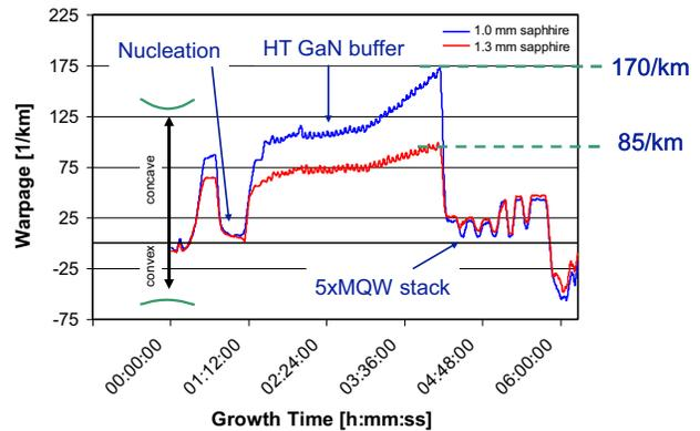
**Figure 4:** Curvature measured using an in-situ deflectometer for a whole MQW process on substrates of different thicknesses
