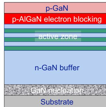
**Figure 1:** Example of a generic LED structure with n-GaN buffer, active zone with multi-quantum well structure, p-type AlGa<sub>x</sub>N electron blocking layer and upper p-GaN.
