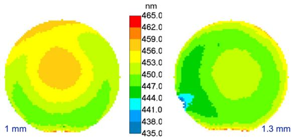
**Figure 5:** PL maps of MQW structures on 6 inch wafers of different thicknesses
