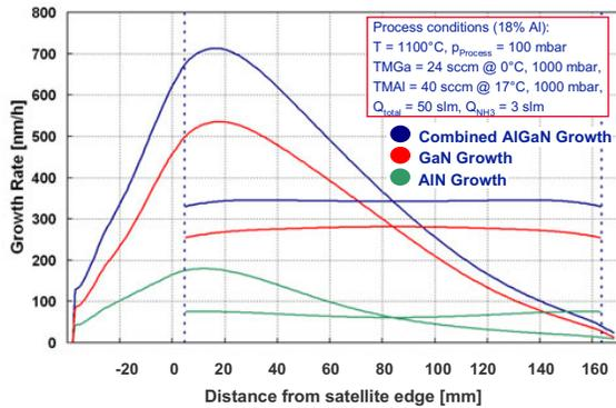
**Figure 2:** Simulation of super-positioning of AlN and GaN for AlGaIn growth
