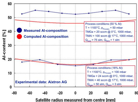
**Figure 3:** Comparison of simulation to experimental data for AlGaIn compositional uniformity across a full 6 inch wafer
